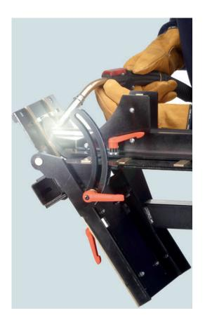
Post welding jig for fast and efficient welding of plates and handrail shells. Whether railing posts, pillars or smaller supports in metalwork: once set up, you can produce individual parts and series parts with the CREA-FIX. Insert components and weld - fast, accurate and efficient.
